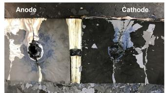
Figure 10: Torn down cell from 200 Wh module following penetration by 2 cm diameter nail.
