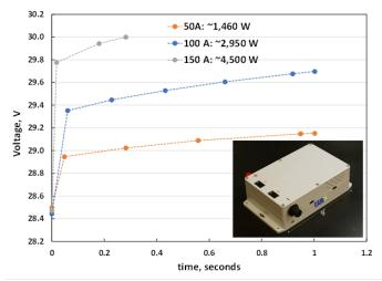
Figure 7: Voltage during constant current charging for 1 sec. or to 30V of CELX-RC-based 2.7 liter, 4.3 Ah, 100 Wh battery module (picture is inset) at indicated currents and corresponding approximate powers, after the module had been charged to 28.5V.
