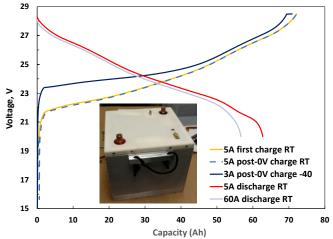
**Figure 4:** Charge and discharge voltage curves for CELX-RC-based 6T battery prototype (picture is inset).
