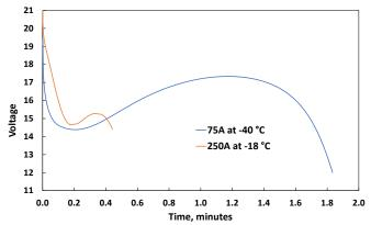
**Figure 8:** 30-second discharge pulsing at -18 °C and 75 A continuous discharge at -40 °C for CELX-RC-based 4.3 Ah battery module.
