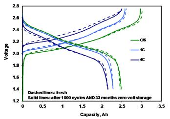
**Figure 1:** Charge and discharge voltage curves at indicated rates for a 2.5 Ah CELX-RC pouch cell before and after 1,000 full cycles at 1C/1C rate and almost 3 years storage in the 0V condition.
