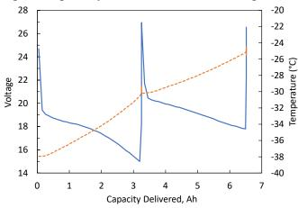
**Figure 5:** Voltage and internal temperature of CELX-RCbased 6T battery prototype at -40 °C as it was discharged at 400 A in two 30-second pulses with 5 minutes intervening rest.
