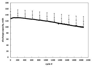
**Figure 3:** Discharge capacity of an unmanaged 11-S stack of CELX-RC pouch cells cycled 28.5 V to 20 V at 200 mA charge and discharge current, with 20, 50 and 100 mA discharges at 200-cycle intervals.
